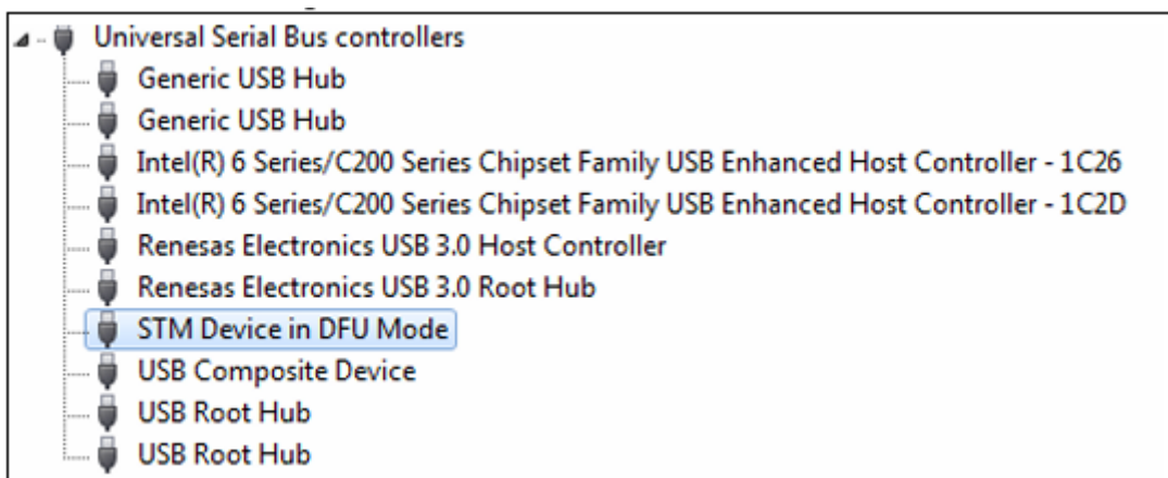
Fig. 2.2: STM32 DFU device with DfuSe driver
