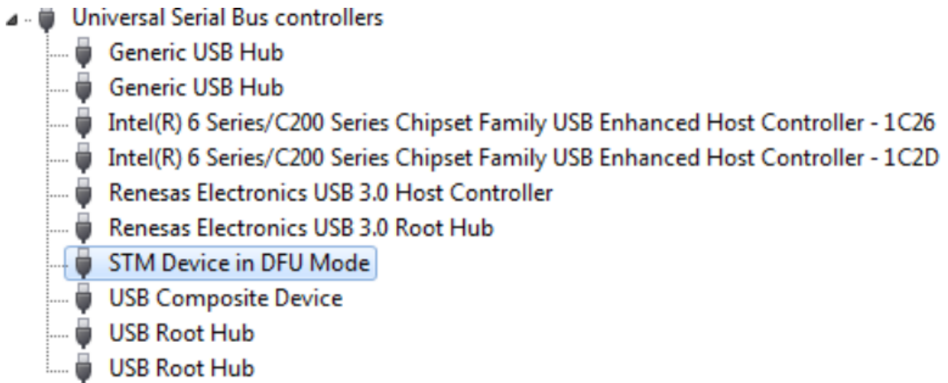
Fig. 4.2: STM32 DFU device with DfuSe driver
