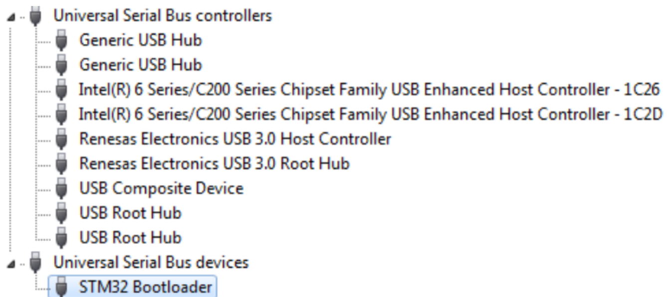
Fig. 4.3: STM32 DFU device with STM32CubeProgrammer driver
